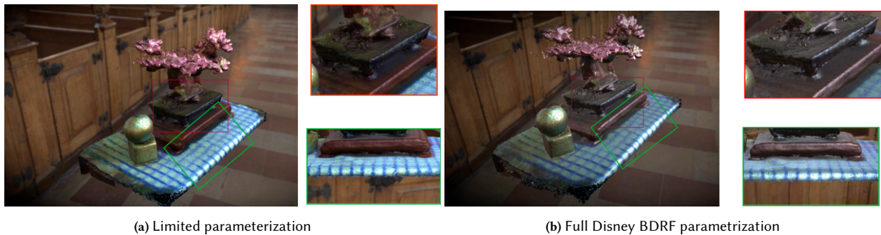
Fig. 11. Optimizing for the full Disney BRDF is difficult. Figure 11a shows our results with only specular, roughness and metallic BRDF parameters. Figure 11b depicts identical results utilizing the complete range of Disney BRDF parameters as outlined in [Cheng et al. 2023]. Note the excessive glossy appearance of Fig. 11b due to the dominance of the clearcoat and clearcoat-gloss parameters. Details in appendix D, meshes rendered with [Sketchfab 2024].
